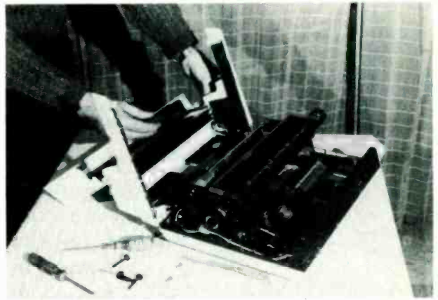
WHEN WORKING ON the Smith-Corona TP-7, you cannot separate the casing top because the leads to the fan are too short.
