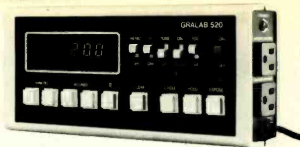
FIG. 2—THE GRALAB 20 DIGITAL DARKROOM TIMER can sound a short tone each second to permit the darkroom worker to carry out time-critical operations like dodging and burning-in without having to watch the time display.
