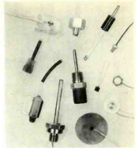
FIG. 11—THERMISTORS AND OTHER temperature sensors are available in a wide variety of sensor assemblies.
