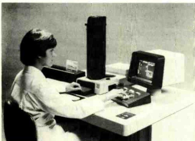
FIG. 6—THIS CONSOLE lets the operator encode information in the disc's magnetic core. That information can be read automatically by special printers.
