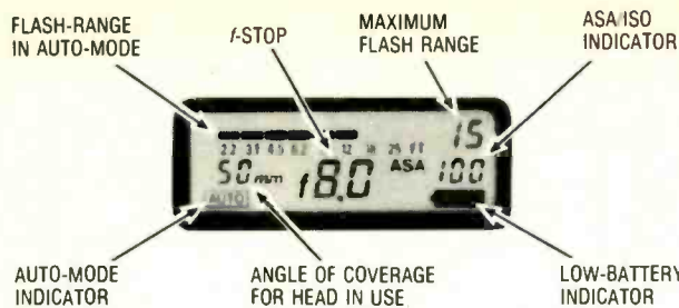
FIG. 3—A CLOSE UP VIEW of the 5600's LCD display shows just how much exposure information it can provide.
